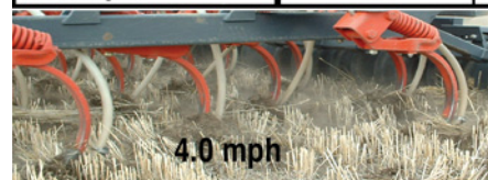
The successful emergence of canola seedlings out of the ground is significantly impacted by the speed at which the seeding operation is carried out.
